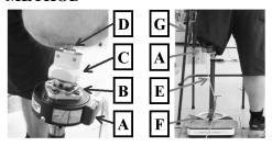
Figure 1. Example of a typical prosthetic leg setup used to directly measure the load applied during load bearing exercises. A commercial transducer (A) was mounted to specially designed plates (B) that were positioned between the adaptor (C) connected to the abutment (D) and the long pylon (E). This setup also included a commercial scale (F), used to monitor the load to be applied and a support frame (G).
