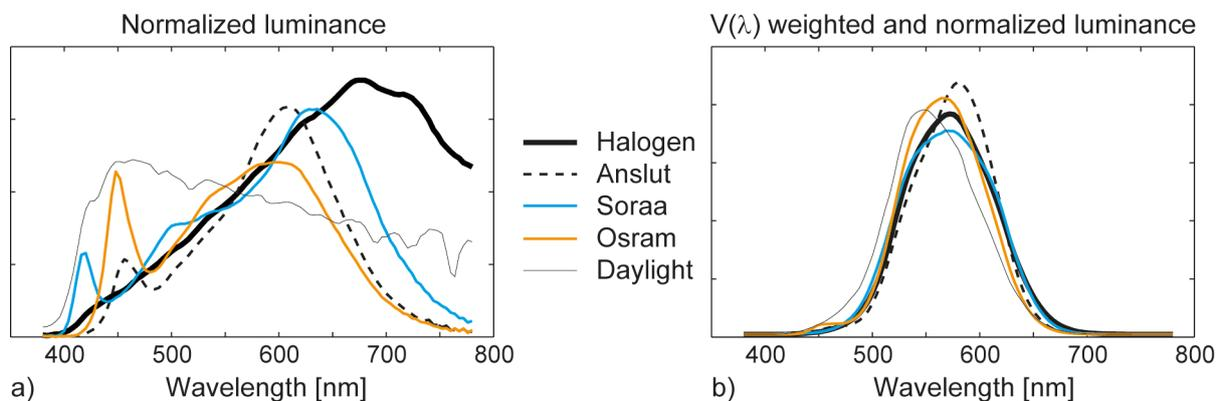
**Figure 3 – SPD of the light sources used in the tests. a) SPD normalized to equal luminance. b) The SPD in a) weighted with  $V(\lambda)$  function.**
